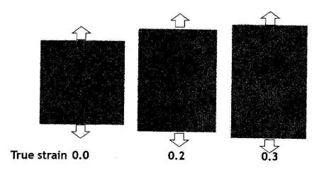
Sequence of snapshots showing the tensile deformation accommodation of a nanostructured alloy. (Ch.E. Lekka et al, J.Nanoscience & Nanotechnology 9(2009)1)
